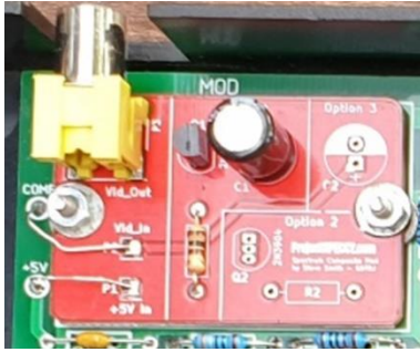
Spectrum 48K Composite Video Mod
